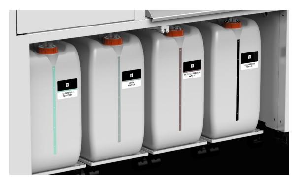
**Large Bulk Containers** The instrument has 2 bottles with a maximum capacity of 25 liters, with the reagents required for the different washing processes. The layout is as follows:
