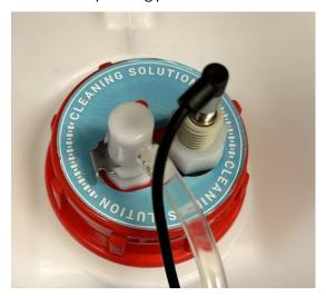
The instrument checks the connection and volume of the bottles before starting a run; if it is not sufficient, an "Insufficient Volume" error is displayed, and if it is not connected, a "Bottle Disconnected" error is displayed. To resolve these issues, you need to connect or replace the large bulk container-and go to the "Troubleshoot Containers" section to resolve the issue at the application level.
