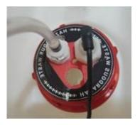
The instrument checks that the waste containers are connected and are not full before starting a run; otherwise, the system will display a "Container disconnected" or "Container Full" error. If the waste container is detected to be full, the final circuit of the container will be automatically emptied to avoid liquid spillage when emptying it. To resolve these issues, connect/replace the container and go to the "Troubleshoot Containers" section for application-level troubleshooting.
