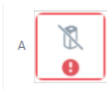
When starting a run or maintenance, and this device is being disabled, the behavior and consequences of disabling the imaging camera are reported in a window.
