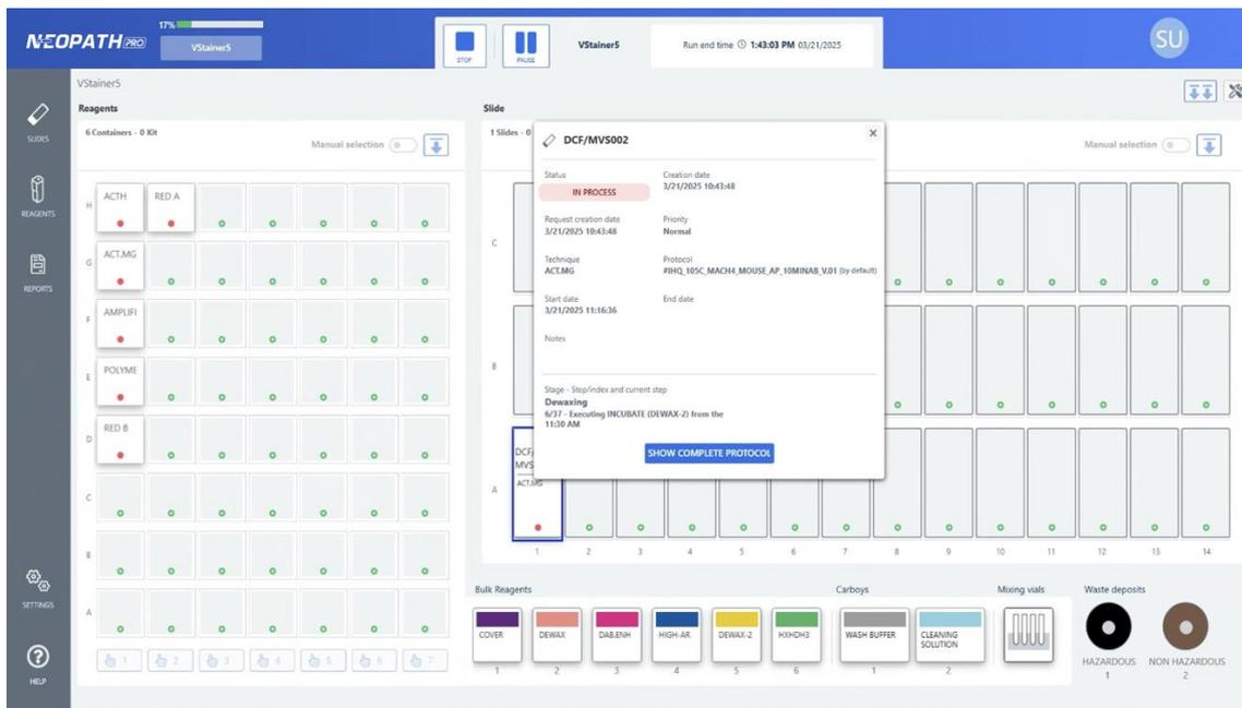
Clicking on each position displays a new window with all of the information corresponding to the status and execution of the slide, so that the user can track the protocol in real time.
