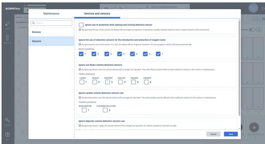
When running a series or maintenance, and the use of the sensor is disabled, it is not reported if a rack is inserted or removed, and all disabled rack positions will be scanned in the reagent vial rack check.
