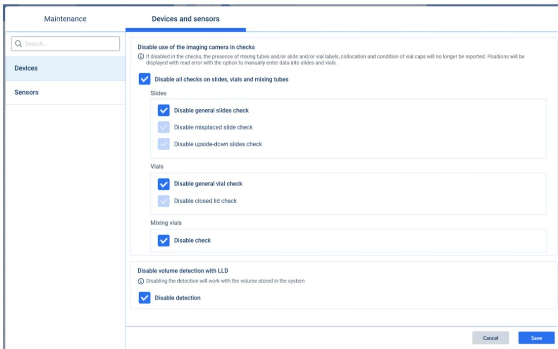
When running a series or maintenance, and the use of the imaging camera is being disabled, the scanning of the port and reagent vial racks is not performed in the port and vial verification, and all positions that were to be read with the imaging camera are represented with not detected error for manual data entry.
