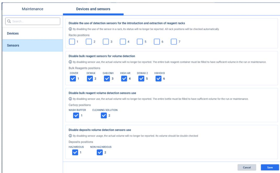
When running a series or maintenance, and the use of the sensor is being ignored, the volume or capacity will not be reported, and should be checked visually, to avoid running a run without sufficient reagent volume or capacity.
