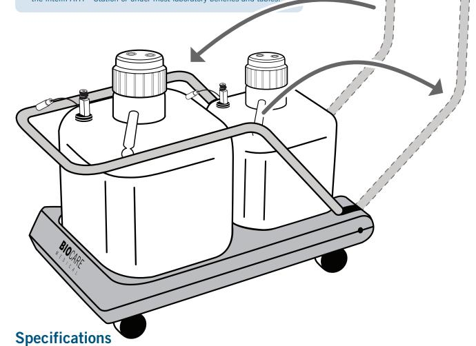
SpecificationsWeight7.2 lbs (empty) / 70 lbs loaded with full carboysDimensions (D x W x H)25.5"x 13.5"x 16.5" (handle closed) / 30.5" (handle open)
